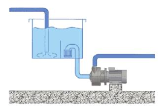
The horizontal centrifugal pumps must only be installed with the axis positioned horizontally in positive suction head. Suitable devices must be used to avoid dry operation, the formation of vortexes and the possible intake of air. The horizontal centrifugal pumps must only operate when the pump is FLOODED; operation when dry or with air bubbles causes damage to the mechanical seal.
